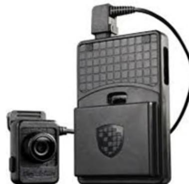
Most operation of the camera is controlled by the officer. The officer will be required to turn on the camera when they arrive on a call. There are features where the camera can automatically turn on. Some have geo-fencing capabilities. For example, we could create a geo-fence around Kohl's. Anytime an officer would enter Kohl's, the camera would automatically turn on. The camera will continue recording until the officer manually turns off the camera.
