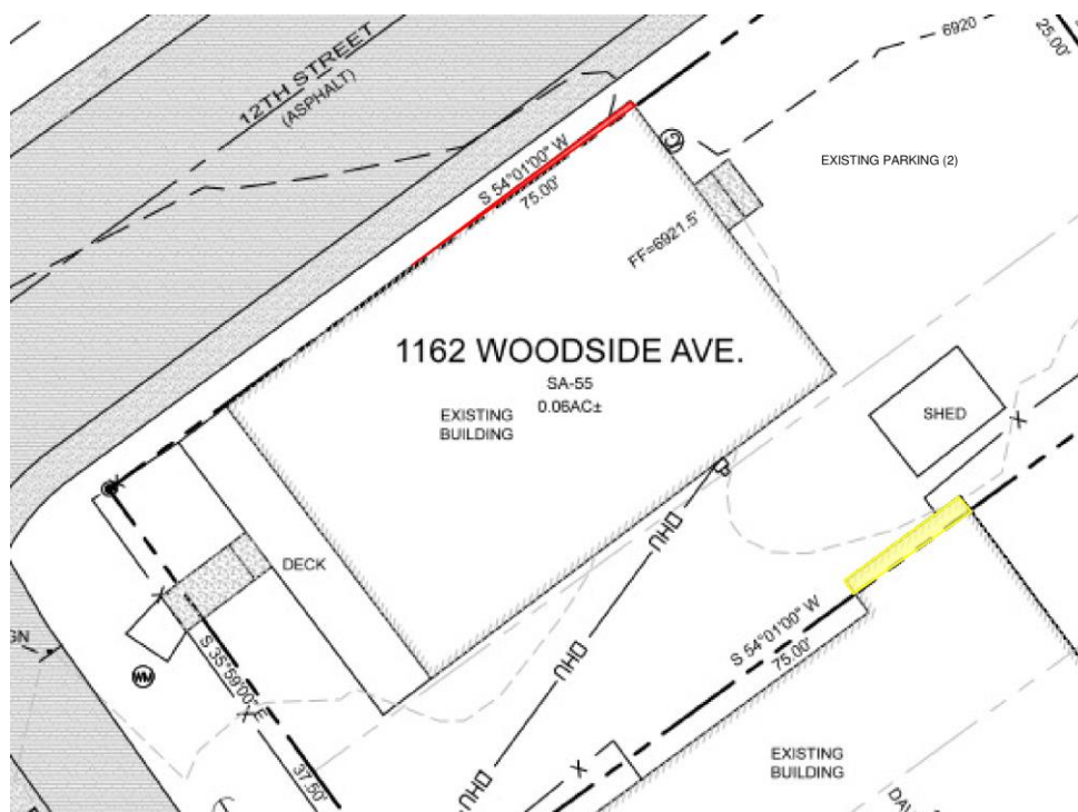
Figure 1: Property survey with encroachments highlighted:
